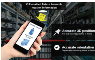
Figure 11: Use of a Smartphone for indoor position location (courtesy of the IEEE and Qualcomm)
