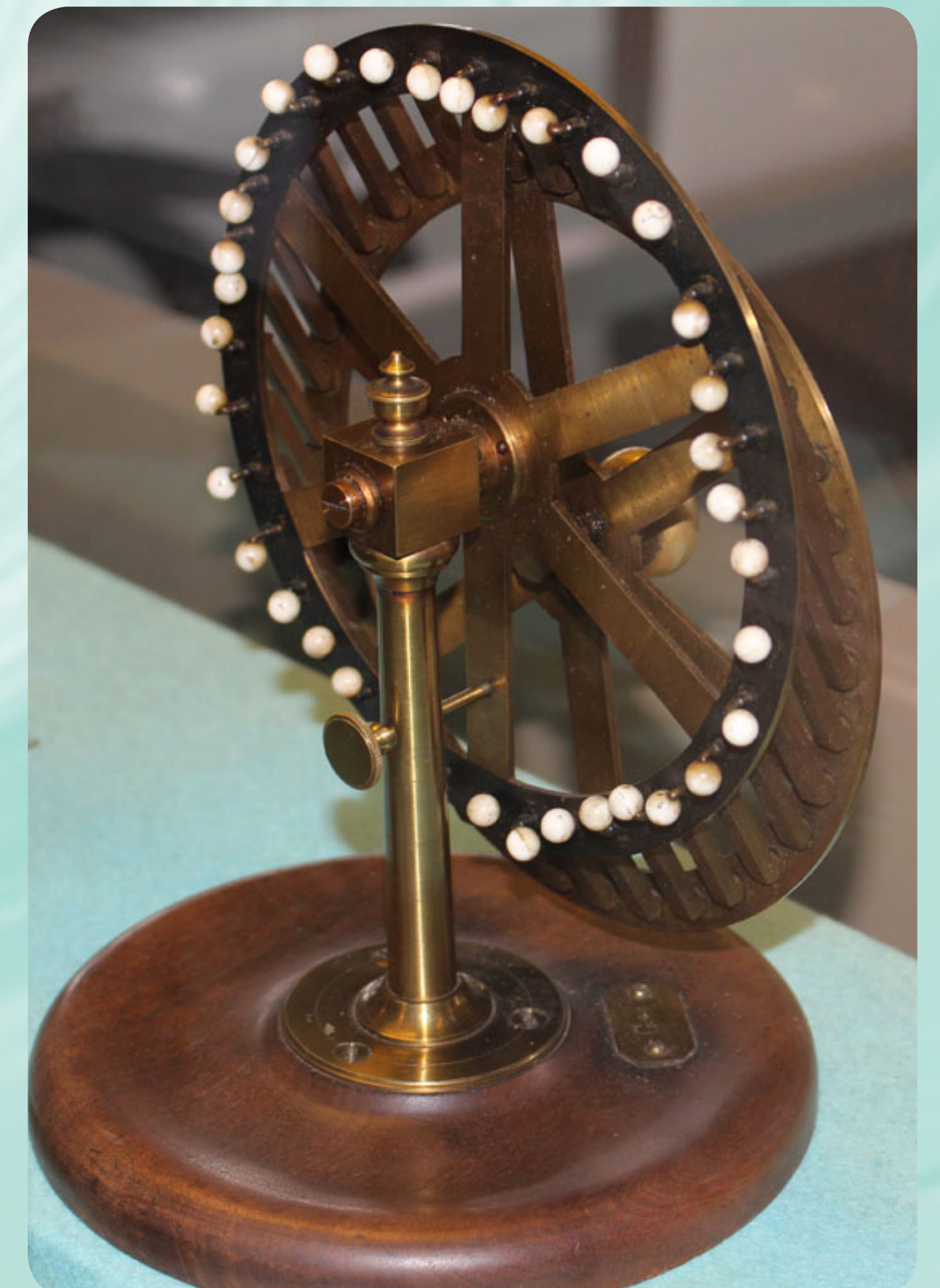
Reproduction of Maxwell's mechanical model of the motion of the individual particles which form the rings of Saturn, courtesy Cavendish Laboratory, Cambridge.
